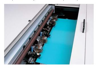
Flatbed imaging system with violet laser diode
