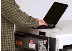
Remote monitoring and diagnostics of the unit or change program settings via ethernet.
