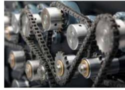
The Gecko<sup>+</sup> 125 uses a traditional chain drive for rollers and brushes.
