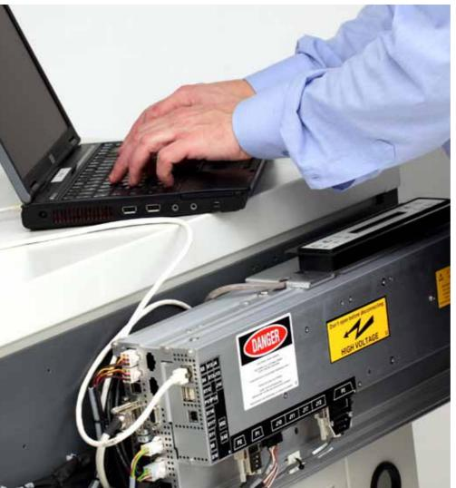
Glunz & Jensen's Remote **Enabling System is** included as standard and is used to configure the processor and allow for convenient remote service access via the internet.
